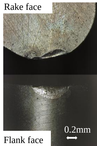
Figure 2. Tool wear of the T4-N coated tool at a substrate DC bias voltage of -300 V and cutting distance of 4.7 km.
