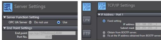
Figure 3. OPCUA setting in Programmable logic controller network.
