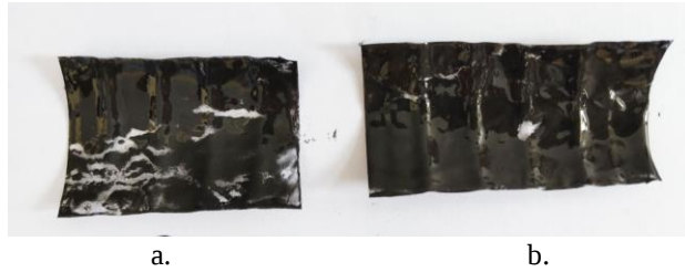
Figure 16 Clumping effect on AMT-Smartech MR fluid when it is used with a. Conventional MR damper and b. modified MR damper
