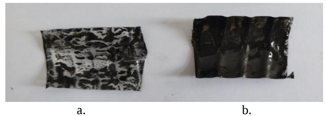
Figure 15. Clumping effect on AMT-Dampro MR fluid when it is used it with a. Conventional MR damper and b. modified MR damper
