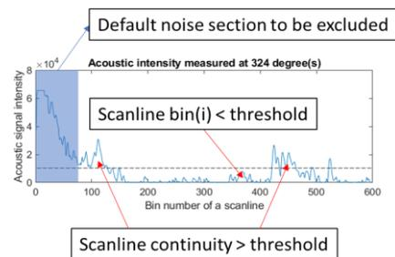
Figure 11. Measurement analysis in dimensional steps. The shaded box in blue indicates that the default noise section was excluded.
