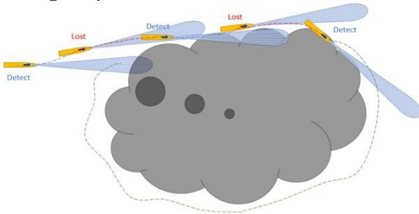
Figure 14. The proposed plume-following motion.
