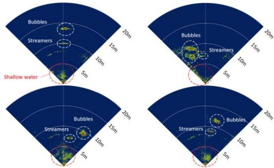
Figure 6. The Ping360 sonar images that captured the micro bubbles and the streamers. Noise reflected from the bottom of the shallower regions of the lake was also detected.
