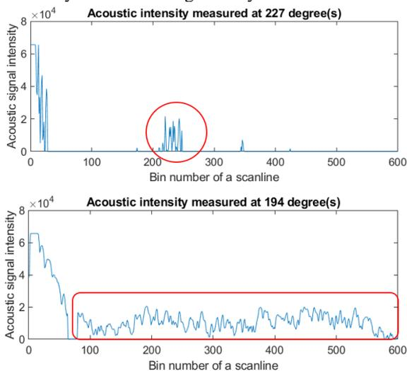
Figure 9. The plots showing a small bubble patch at a range of 20m (*top*) and a longer trail of bubbles at a range of 5m (*bottom*), respectively.
