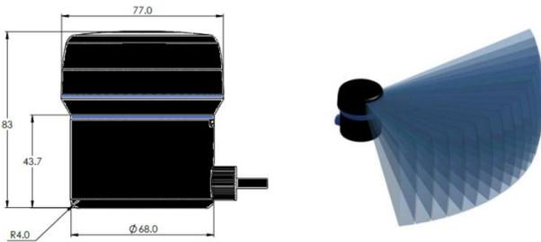
Figure 3. Ping360 Scanning sonar (left); Scanning coverage (right).
