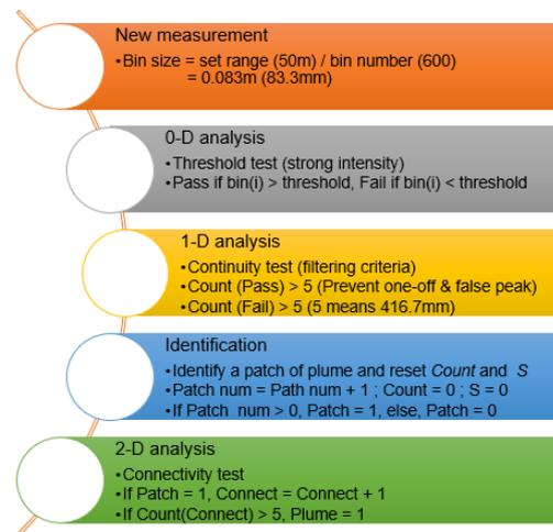
Figure 12. The pseudo code for real-time analysis of in-situ acoustic intensity measurements.
