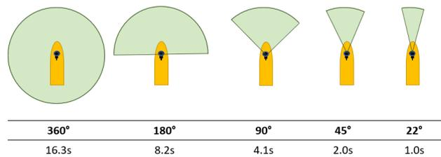
Figure 13. Required time for varied scanning sector at a 15m range.
