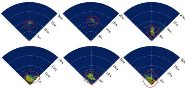
Figure 7. The Ping360 sonar images of the air bubbles during the Lake Barrington tests. The target is shown at different distances from the sonar head.
