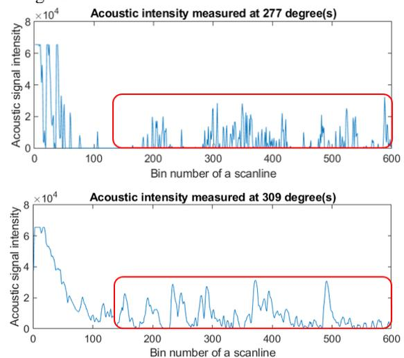
Figure 10. Plots showing different trends in multiple patches: a noisy plume (*top*) at a bearing angle of 277° and a relatively less noisy plume (*bottom*) at a bearing angle of 309°, respectively.
