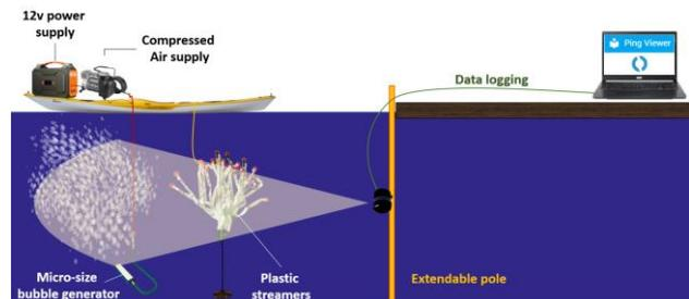
Figure 5. A schematic diagram of the test site in Lake Barrington (Not to scale).
