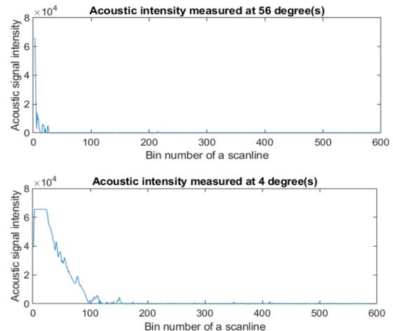
Figure 8. The plots showing 1-D acoustic measurements at a bearing angle of 56 ° with a range of 20m (top) and 4 ° with a range of 5m (bottom), respectively.
