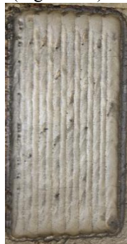
Figure 19. Cladding test area using Powder System 2
