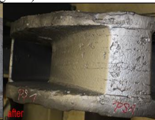
Figure 3. Impeller, after cleaning by blasting with steel chips
