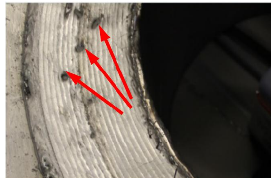
Figure 24. Cladding of cover plate (pores in the coating)
