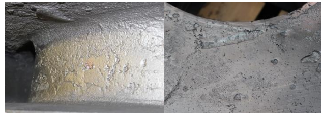
Figure 6. After blasting, impeller surface
