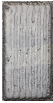
Figure 20. Cladding test area using Powder System 2
