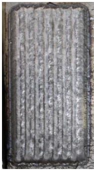
Figure 18. Cladding test area using Powder System 1
