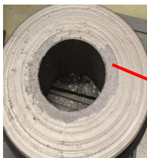
Figure 25. Removed laser cladding at inner area
