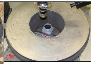
Figure 5. Cover plate, after cleaning by blasting with steel chips
