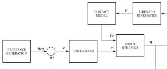
Figure 3. Simulation environment block diagram.
