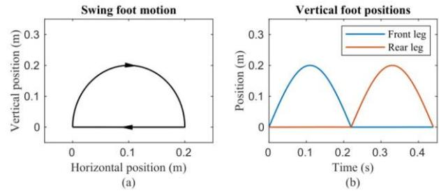
Figure 4. Foot positions in one cycle, (a) foot motion in space, (b) vertical foot position in time.
