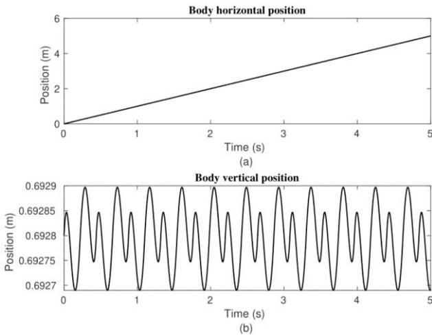
Figure 6. Body linear positions, (a) horizontal position, (b) vertical position.
