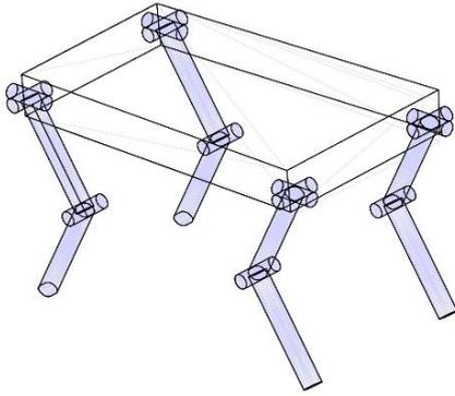
Figure 2. Kinematic arrangement of the detailed quadruped robot.
