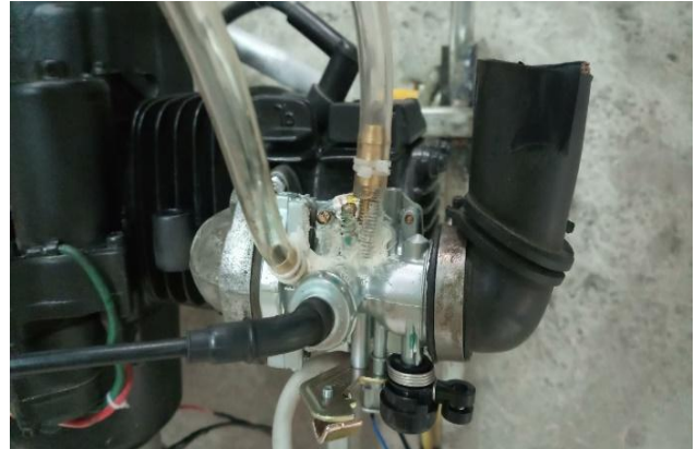
Figure 3. The engine uses bi-fuel CNG and gasoline, the carburetor with two holes are drills to push CNG into the mixer.
