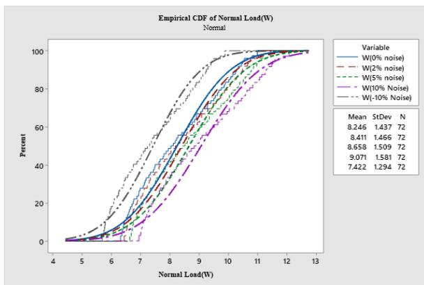
Figure 15. Empirical Cumulative Distribution Function (CDF) of normal load at different noise levels
