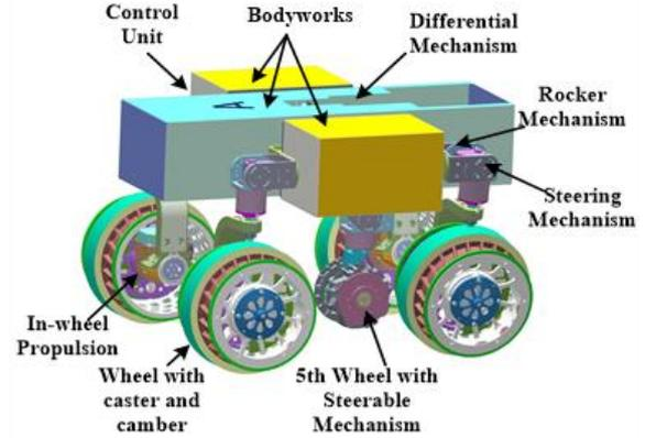
Figure 2. Pro/E model of autonomous vehicle
