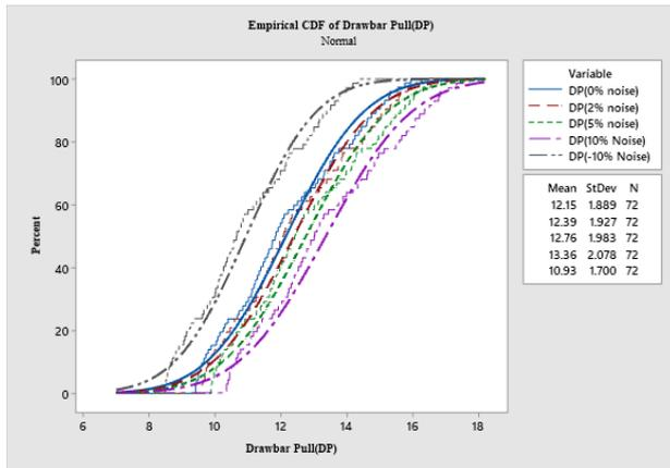
Figure 14. Empirical Cumulative Distribution Function(CDF) of drawbar pull at different noise levels
