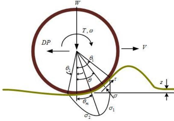
Figure 3. Rigid wheels on deformable terrain.
