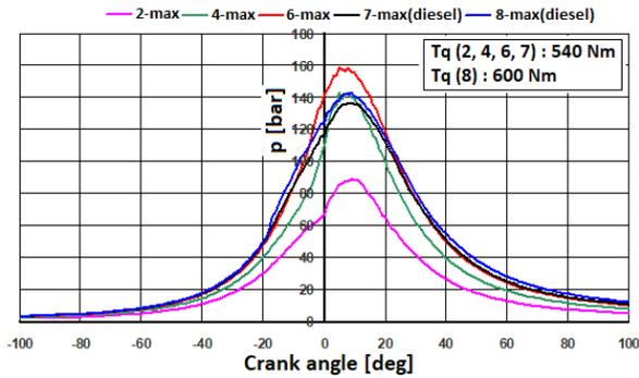
Figure 20. Cylinder pressure curves in the DF mode at the engine speed of 2300 rpm.
