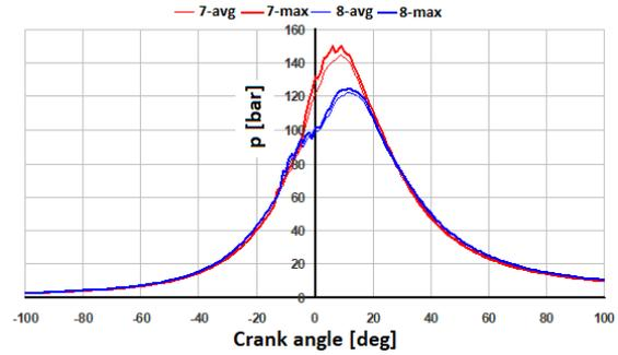
Figure 21. Comparison of cylinder pressure curves for n=1500 rpm and Tq=600 NM when engine running on diesel (No. 8) and in DF (No.7) operation.
