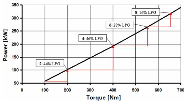
Figure 13. Engine heat input at the engine speed of 1900 rpm: diesel and LPG shares in the DF mode.
