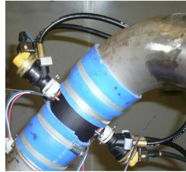
Figure 4. Installation of the LPG injectors into the intake pipe.
