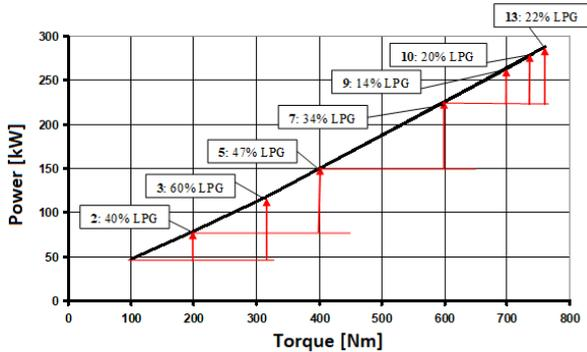
Figure 12. Engine heat input at the engine speed of 1500 rpm: diesel and LPG shares in the DF mode.
