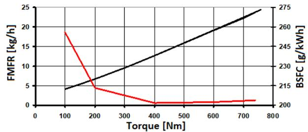
Figure 9. Diesel fuel consumption at the engine speed of 1500 rpm.
