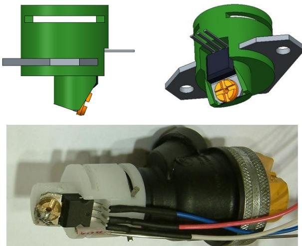
Figure 3. The assembly of the electromagnetic injector and its end part with the heated outlet nozzle.
