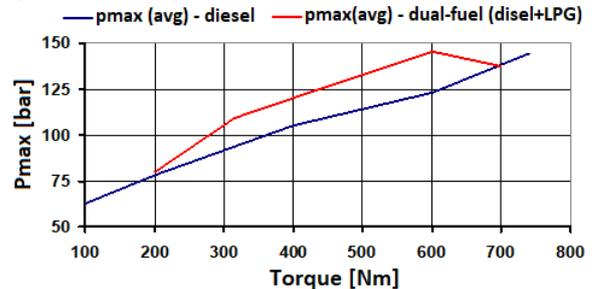
Figure 15. Maximal combustion pressure curves at the engine speed of 1500 rpm.
