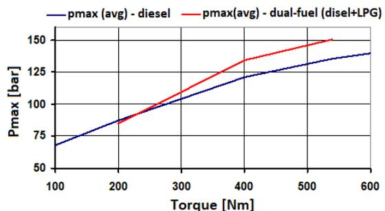
Figure 17. Maximal combustion pressure curves at the engine speed of 2300 rpm.
