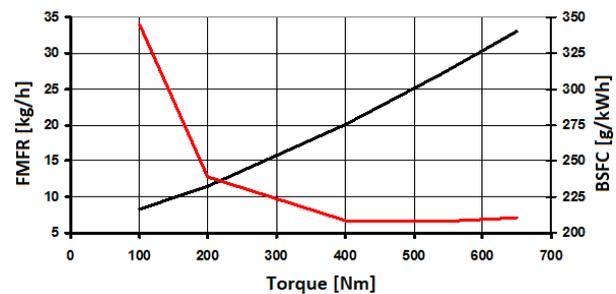
Figure 11. Diesel fuel consumption at the engine speed of 2300 rpm.
