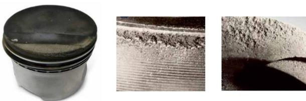
Figure 2. Piston damage due to high heat transfer (erosion on the crown of the piston) caused by knocking.
