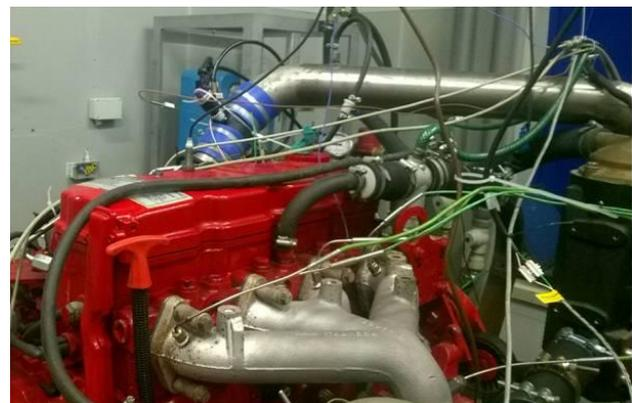
Figure 6. Gas DF engine Cummins with an injection of liquid LPG into the intake manifold.
