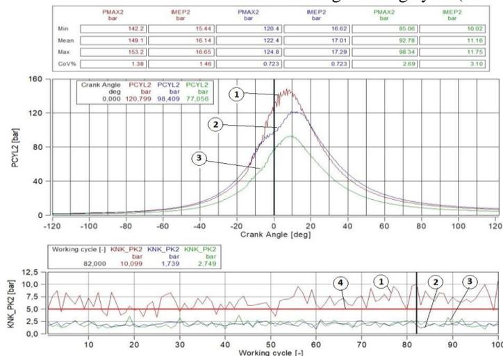
Figure 22. Comparison of a knock when engine running on diesel and DF operation.
