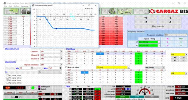
Figure 5. Monitor with S.W. electronic control units Solaris LPG-diesel.
