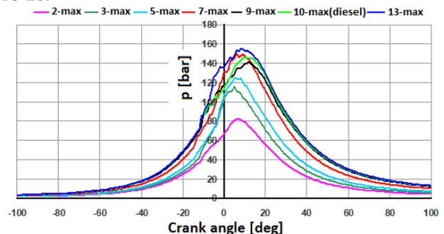
Figure 18. Cylinder pressure curves in the DF mode for engine speed 1500 rpm.
