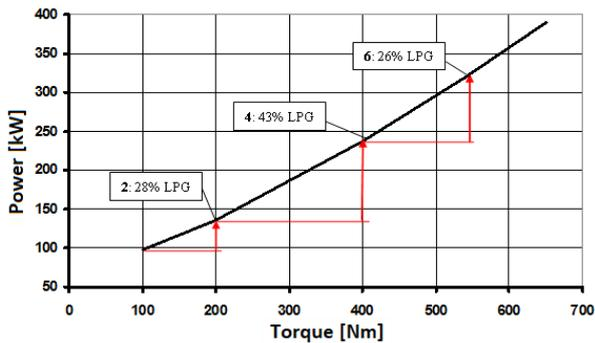
Figure 14. Engine heat input at the engine speed of 2300 rpm: diesel and LPG shares in the DF mode.
