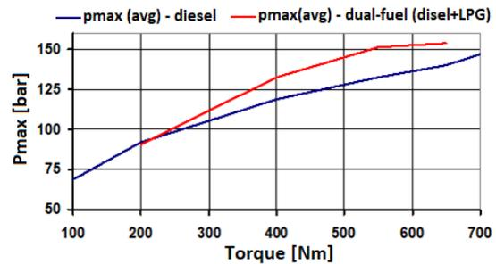
Figure 16. Maximal combustion pressure curves at the engine speed of 1900 rpm.
