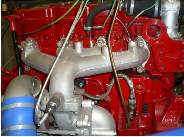
Figure 7. Gas DF engine Cummins view of engine exhaust.
