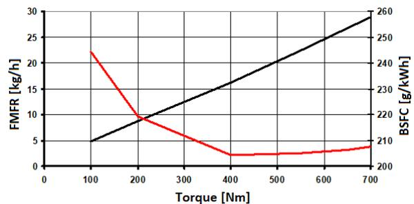
Figure 10. Diesel fuel consumption at the engine speed of 1900 rpm.
