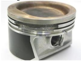
Figure 1. Piston damage due to pressure oscillations caused by knocking.
