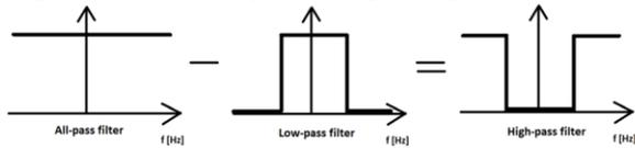
Figure 8. Splitting of the signal parts obtained from the knock sensor.
