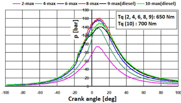
Figure 19. Cylinder pressure curves in the DF mode at the engine speed of 1900 rpm.
