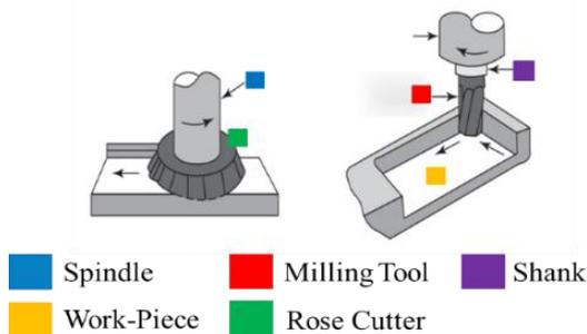
Figure 1. The schematic representation of the milling process
