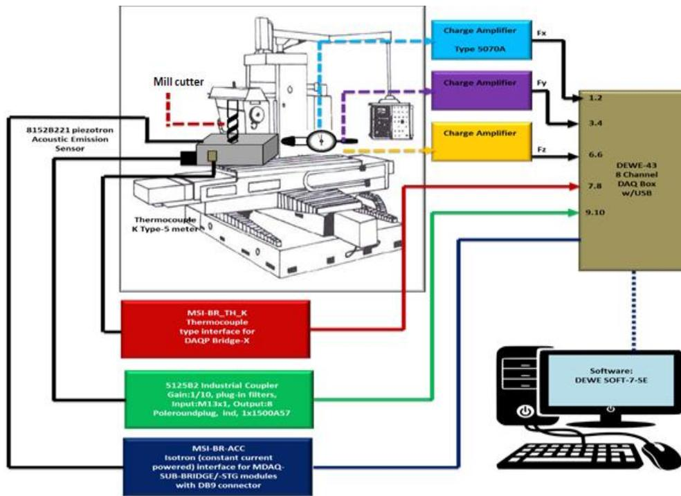
Figure 2. The schematic of the experimental set up and the DAQ.
