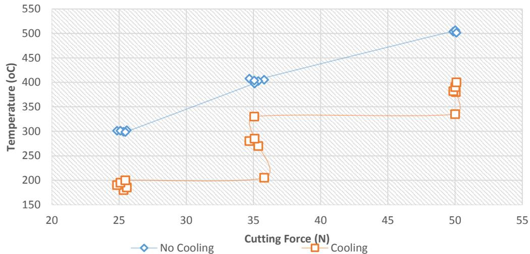
Figure 11. Cutting force-temperature relationship under cooling and dry machining conditions.
