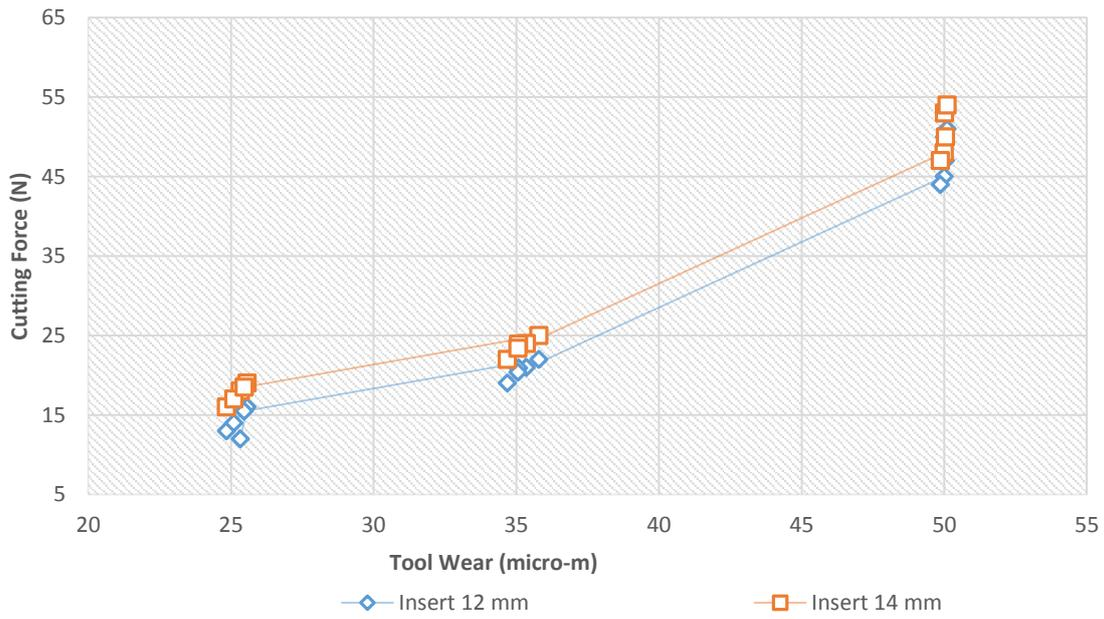
Figure 8. The wear rate using different inserts under cooling conditions.
