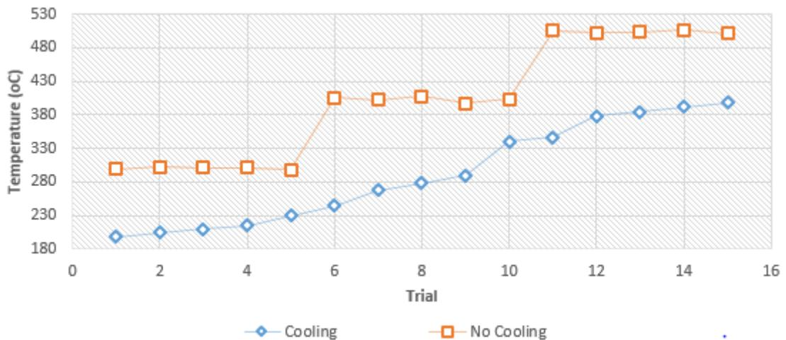
Figure 10. The temperature profile under cooling and dry machining conditions.
