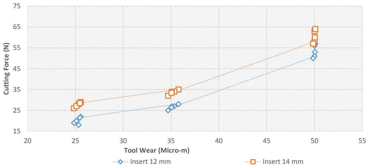
Figure 9. The wear rate using different inserts under dry machining conditions.
