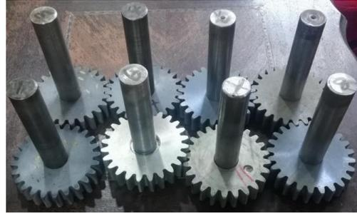
Figure 5. Assembled shaft and gear specimens.
