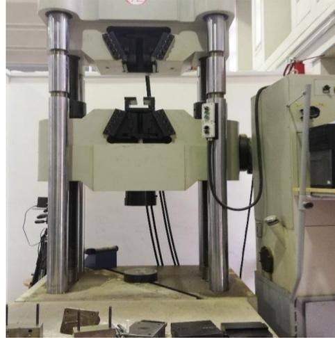
Figure 6. A universal tensile testing machine.
