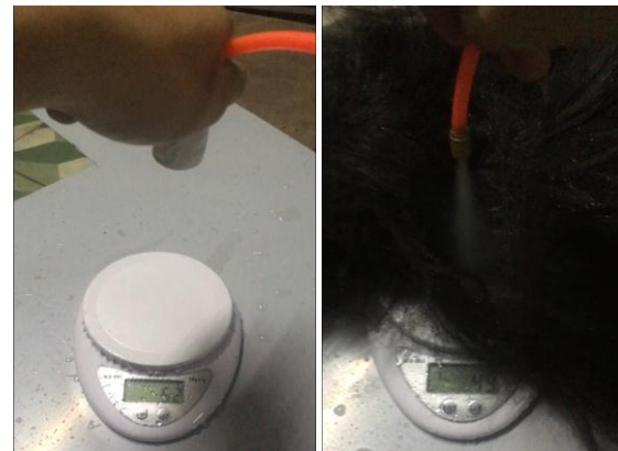
Figure 9. Water nozzle with high pressure (13Psi), jetting directly on the dynamic weight scale surface (left) and jetting on the scales surface through hair resistance (right)
