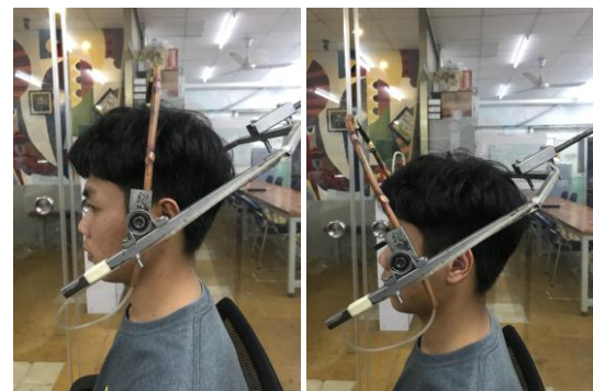
Figure 8. Water jet nozzles, integrated on rotation ring was performed the trajectories to generate scalp wash and massage on the real man
