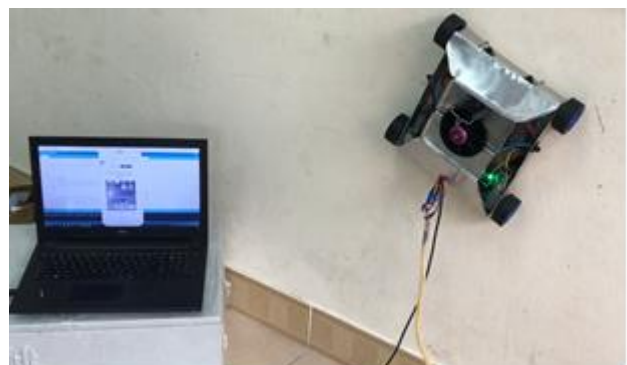
Figure 9. WCR on the wall.
