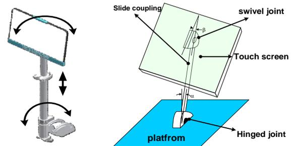
Figure 4. Designed for pan and tilt, holding touch screen and navigation camera
