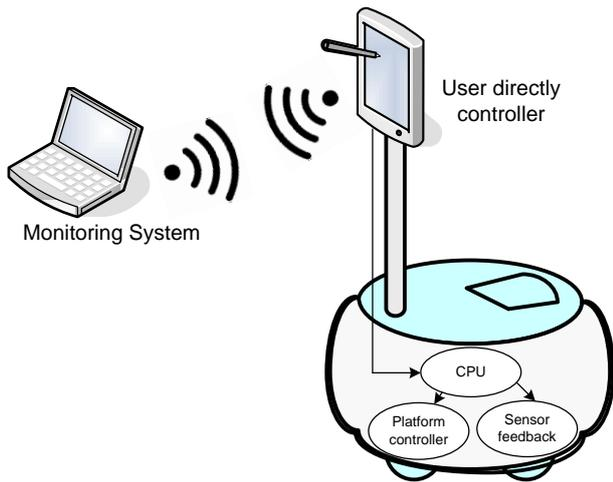
Figure 5. Monitor system (Personal Computer) control robot via wireless connection
