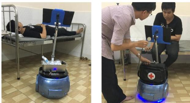
Figure 8. Robot is carrying specimens of patient (left) – robot annual checking patient and report to doctor about patient's condition (right)
