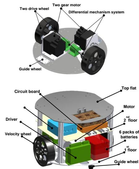
Figure 2. Telemedicine is using differential gear for autonomous platform with two floors design that contained all complex control system.
