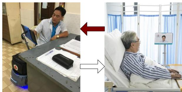
Figure 9. Robot is connecting doctor and patient in different places by video conferencing in real-time
