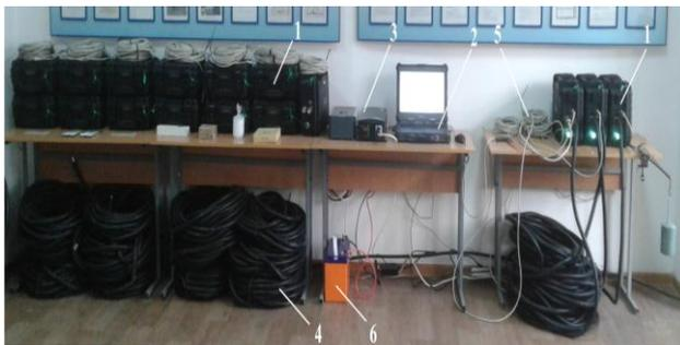
Figure 1. Tens metric measuring and computing complex for measuring relative deformations and stresses in structures: 1 – measuring modules (16 pieces); 2 – semi-industrial laptop; 3 – sinusoidal inverter; 4 – intermodulation connection cable; 5 – connecting cable between the measuring module and the primary transducer (strain gage); 6 – accumulator battery.
