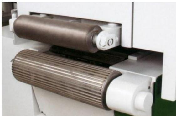
Figure 3. An auxiliary power wheel
