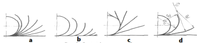
Figure 3. Schemes of tube forming: a - bending with a constant radius; b - bending from the edges to the middle of the strip; c — bending from the middle to the edges of the strip; d — bending using conjugate radiuses
