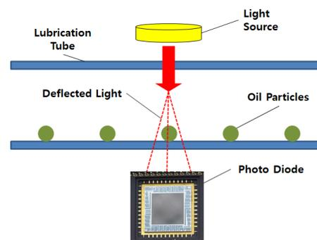
Figure 2. Oil mist lubrication sensor theory.
