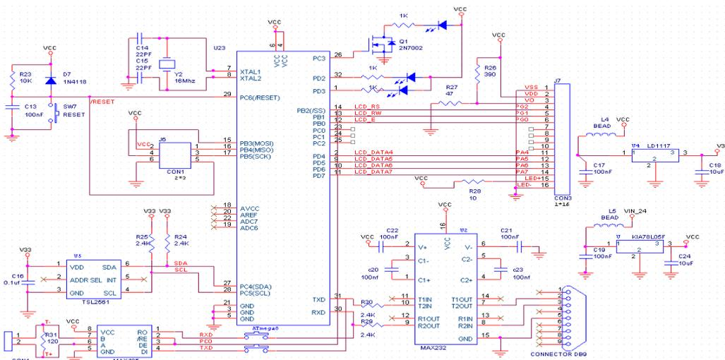
Figure 13. The manufactured oil mist lubrication sensor circuit.
