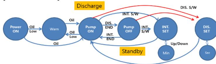
Figure 4. Lubrication pump control state diagram.
