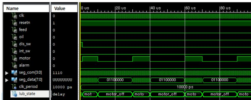
Figure 6. Lubrication IP motor\_on/off.
