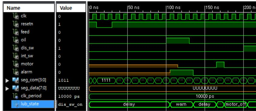
Figure 5. Lubrication IP initialization.
