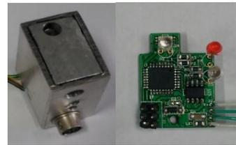
Figure 12. a) Oil mist lubrication sensor & PCB
