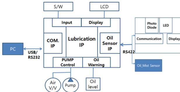
Figure 3. Block diagram of oil mist lubrication.
