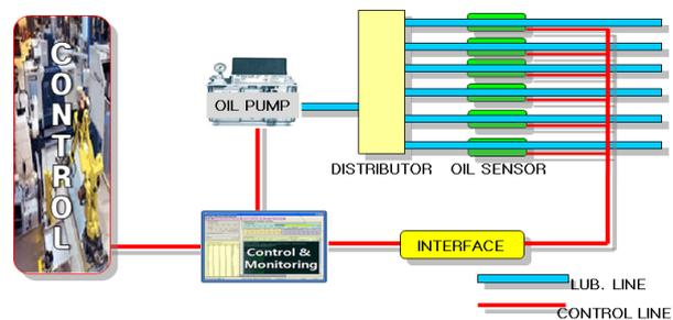
Figure 1. Oil mist lubrication system.
