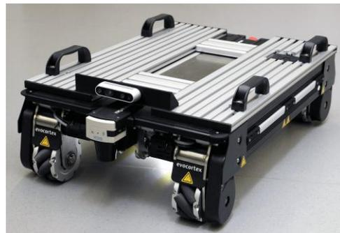
Figure 1. Mobile research platform from evocortex GmbH, Nuremberg, Germany [25]
