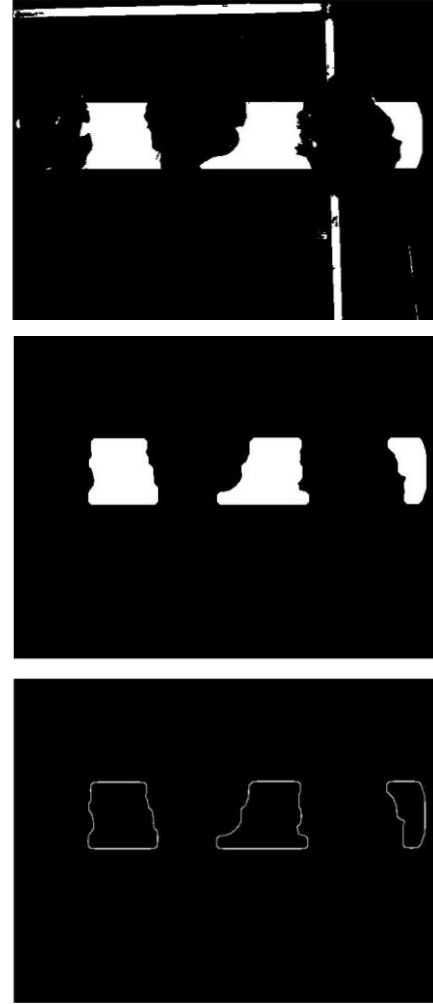
Figure 7. Images after segmentation (top), hole filling and morphological open (middle) and Canny edge detection (bottom).
