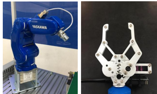
Figure 8. Yaskawa 6 DOF MotoMini manipulator (left) and servo controlled gripper (right).
