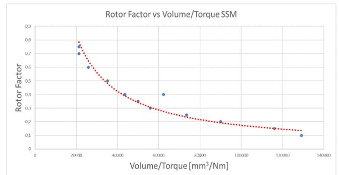
Figure 6. Rotor factor SSM
