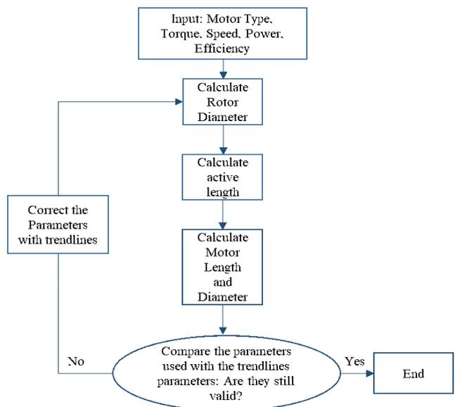
Figure 13. Proposed designing method flowchart
