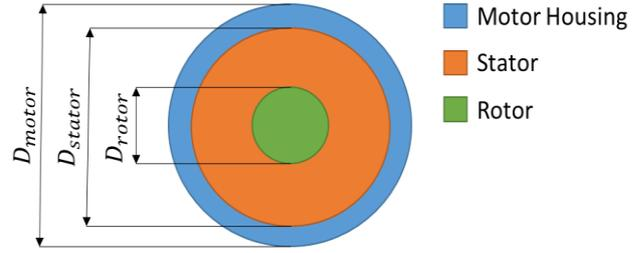
Figure 8. Model of the motor
