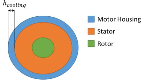
Figure 7. Cooling height and the stator diameter
