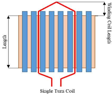
Figure 9. Winding coil length
