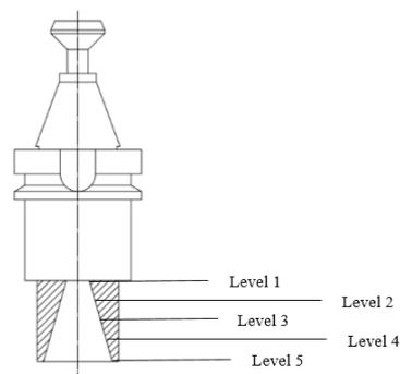
Figure 10. Division of tool holder across its taper length.
