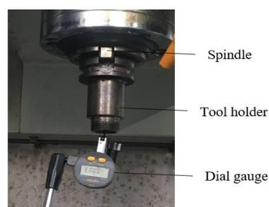
Figure 11. Measurement setup for tool holder.
