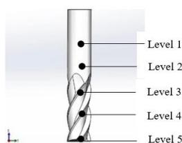
Figure 14. Division of milling cutter across the parallel surface length.
