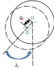
Figure 1. Offset magnitude vector  $e_c$  and location angle vector  $\lambda_c$ .
