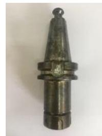
Figure 4. BT40/ER25\*100H (G2.5 20000RPM).
