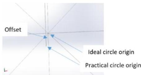
Figure 17. Finding of offset for level 1 of tool holder at 180°
