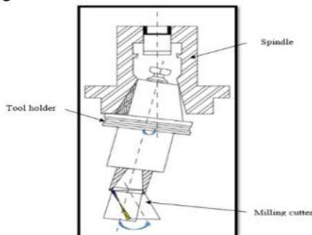
Figure 2. Section view of 2-D model exhibiting eccentric errors
