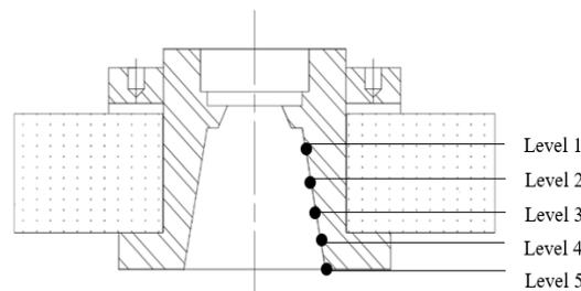
Figure 9. Section view of internal taper length surface of spindle
