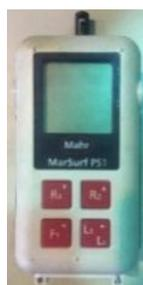
Figure 7. Surface roughness tester MarSurf PS1.
