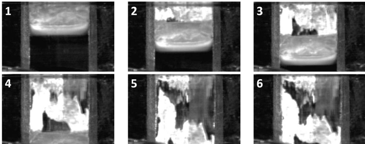
Figure 7. High-speed recordings of the stamping process with transparent insert show film formation and propagation.
