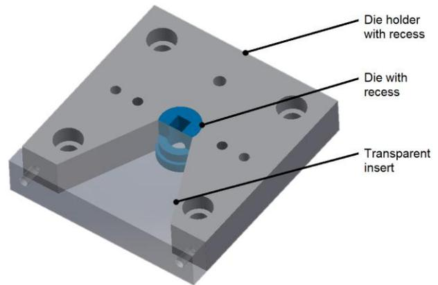
Figure 4. Cutting die and corresponding holder each with recess.
