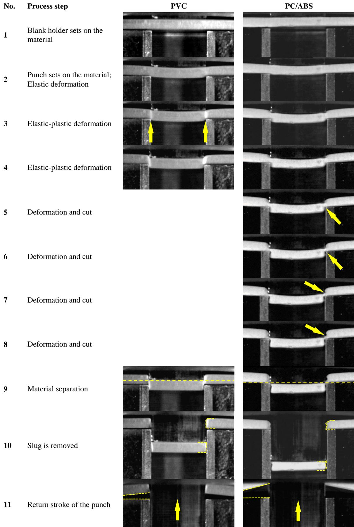
Figure 6. High-speed recordings of the characteristics of PVC and PC/ABS while punching.
