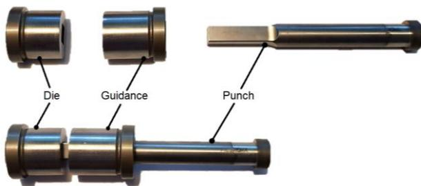
Figure 3. Active elements of the transparent tool.
