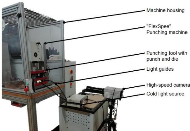
Figure 2. Experimental set-up for the high-speed recordings of the punching process.
