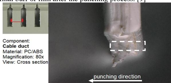
Figure 1. Falsification of burr and film formation on the component bend against punching direction due to the return stroke of the punch [9].
