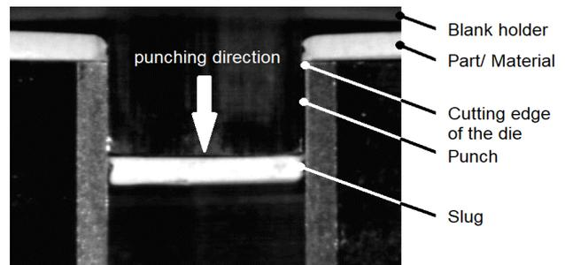
Figure 5. Display of the elements visible in the high-speed recordings.
