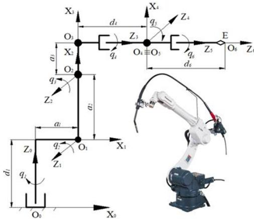
Figure 1. Kinematics model of the welding robot TA 1400
