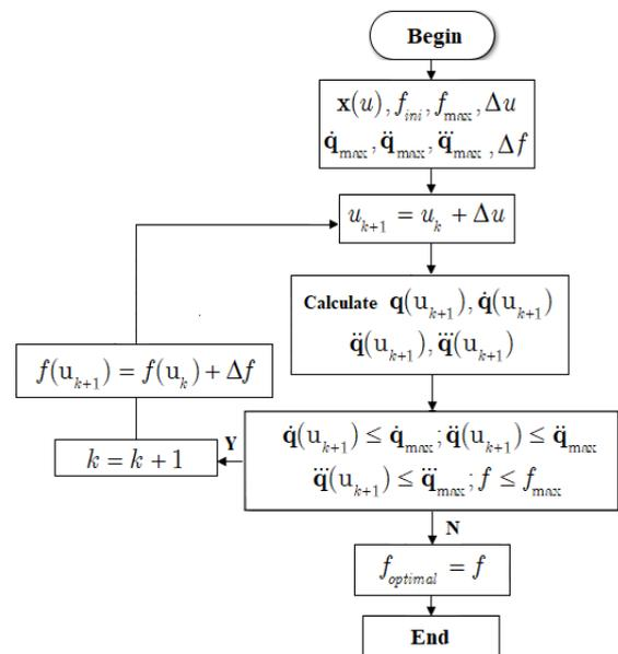
Figure 2. The algorithm diagram for feed rate optimization
