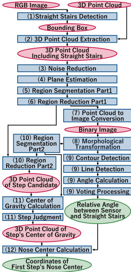
Figure 1. The processing flow of estimating the position and orientation of stairs.
