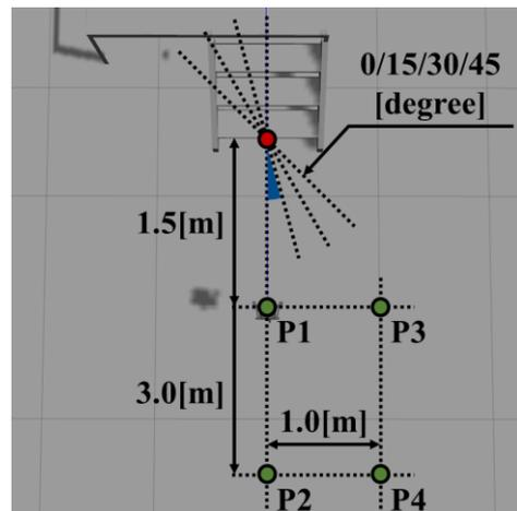
Figure 15. The pattern of the position and orientation of the stairs. Red point: The position of the stairs. Green points: The positions of Multisense SL. (P1-P4: Position1-Position4). Blue ranges: The orientations of the stairs. (0-45: Orientation0-Orientiaon45).
