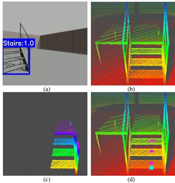
Figure 16. The estimation of the position of the stairs in "Stairs with handrails/Position3/Orientation45". (a) Detection using SSD. (b) A 3D point cloud acquired by Lidar. (c) A 3D point cloud that includes the stairs extracted by Frustum Culling. (d) A 3D point cloud in which the position of the stairs and the representative point of the step are superimposed on (b).
