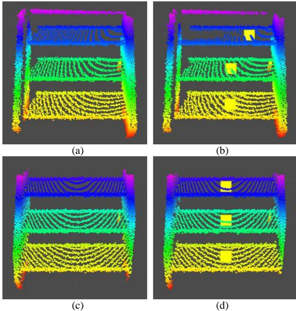
Figure 17. Noise removal using Statistical Outlier Removal. (a)(b) An example of applying to stairs without handrails at Position2 and Orientation30. (c)(d) An example of applying to stairs without handrails at Position2 and Orientation0. (a)(c) A 3D point cloud including the stairs extracted by Frustum Culling. (b)(d) A 3D point cloud from which noise has been removed by Statistical Outlier Removal.
