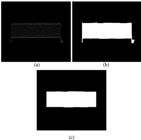
Figure 10. Noise removal using morphological transformation. (a) A generated binary image. (b) Noise removal by closing. (c) Noise removal by opening.
