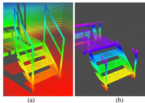
Figure 4. Extraction of 3D point cloud including stairs using frustum culling. (a) A 3D point cloud acquired by Lidar. (b) A 3D point cloud that includes the stairs extracted by Frustum Culling.
