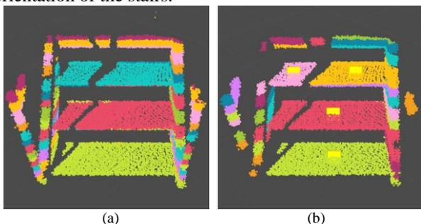
Figure 19. Segmentation of the region using Euclidean Clustering to "the stairs with handrails / Position1 / Orientation45". (a) A 3D point cloud of the step candidate extracted by RANSAC. (b) A 3D point cloud of the step candidate divided by Euclidean Clustering.
