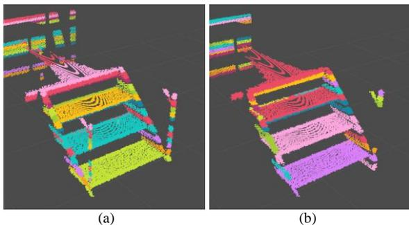
Figure 7. Region segmentation using Euclidean Clustering. (a) A 3D point cloud of the step candidate extracted by RANSAC. (b) A 3D point cloud of the step candidate divided by Euclidean Clustering.
