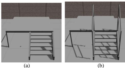
Figure 2. Stairs used for experiments. (a) Without handrails (b) With handrails.
