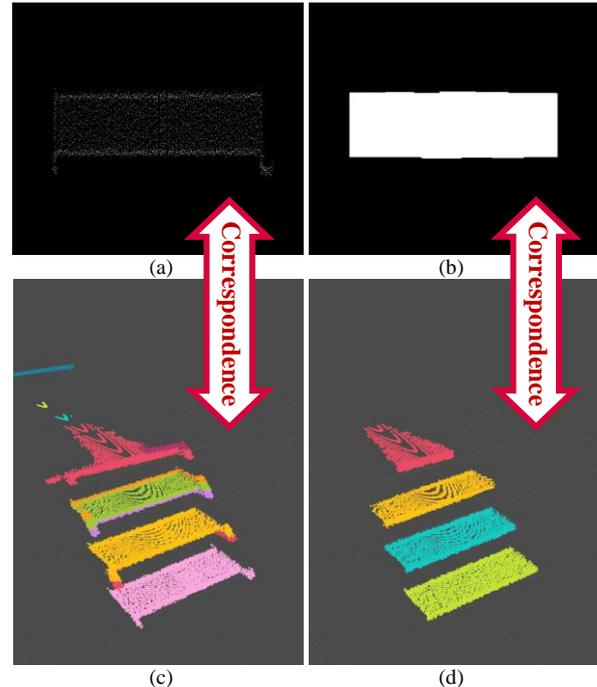
Figure 12. Region removal based on comparison between binary image and 3D point cloud. (a) A generated binary image. (b) A binary image from which noise has been removed by opening. (c) A 3D point cloud obtained by removing the region based on the normal vector. (d) A 3D point cloud obtained by removing the region based on the comparison between the binary image and the 3D point cloud. The white pixels in (a) and (b) correspond to the 3D point clouds in (c) and (d).
