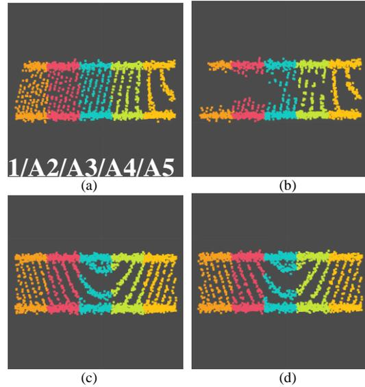
Figure 18. Noise removal using Statistical Outlier Removal to the 3D point cloud of the third step. (a)(b) An example of applying to stairs without handrails at Position2 and Orientation30. (c)(d) An example of applying to stairs without handrails at Position2 and Orientation0. (a)(c) A 3D point cloud including the stairs extracted by Frustum Culling. (b)(d) A 3D point cloud from which noise has been removed by Statistical Outlier Removal.
