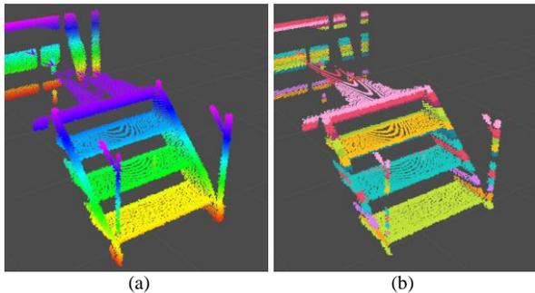
Figure 6. Plane estimation using RANSAC. (a) A 3D point cloud from which noise has been removed by Statistical Outlier Removal. (b) A 3D point cloud of the step candidate extracted by RANSAC.
