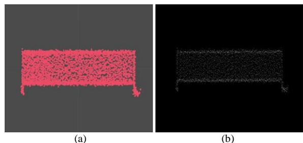
Figure 9. Generation of binary image of 3D point cloud using projection processing. (a) A 3D point cloud of the step candidate projected on a horizontal plane. (b) A binary image generated by plotting (a).
