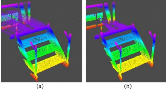
Figure 5. Noise removal using Statistical Outlier Removal. (a) A 3D point cloud that includes the stairs extracted by Frustum Culling. (b) A 3D point cloud from which noise has been removed by Statistical Outlier Removal.
