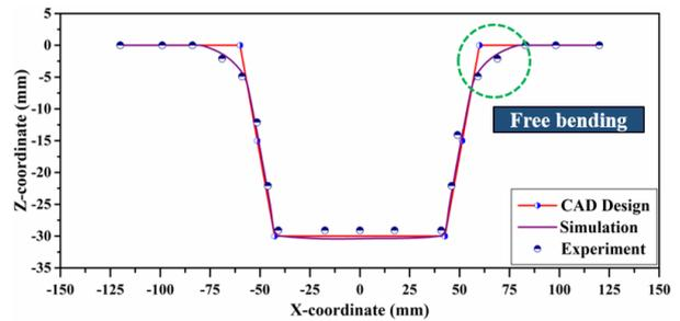
Figure 8. Shape comparison against the experiments (60° angle).
