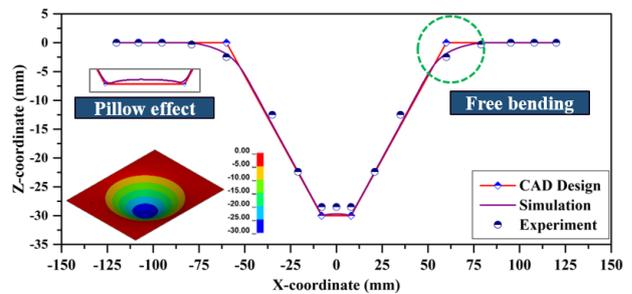
Figure 6. Shape comparison against the experiments (30° angle).
