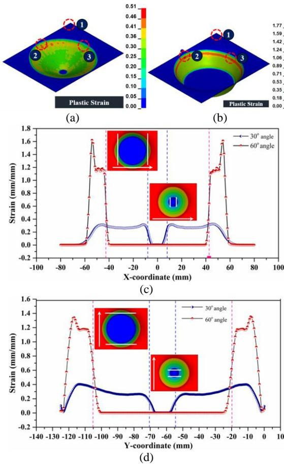
Figure 10. Strain variations in simulated part.
