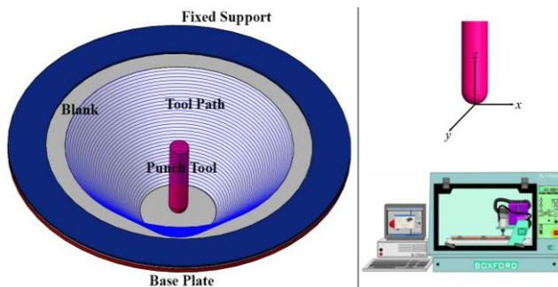
Figure 1. Schematic diagram of SPIF process.
