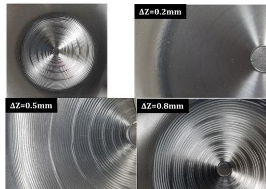
Figure 3. Surface roughness (formed cone shape).
