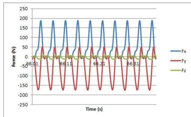
Figure 1. Ten periods of cutting force components in the hard milling
