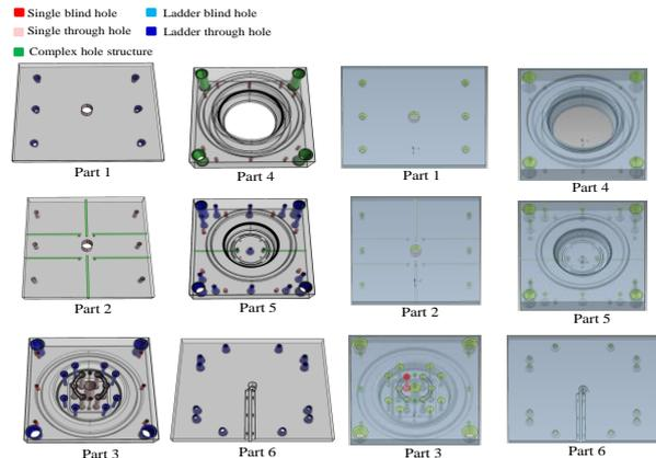
Figure 12. Results of hole recognition for Case 2, where left and right panels denote the proposed method and CADdoctor, respectively.
