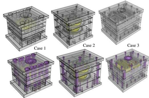
Figure 11. Three injection molds used in this study, where left plots indicate the original CAD models and right plots indicate the results of hole recognition.
