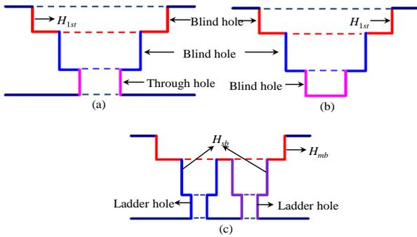
Figure 6. Various structures of ladder holes: (a) a ladder hole with a through face on the bottom, (b) a ladder hole with a blind face on the bottom, and (c) a hole that connects to multiple parallel holes is excluded from the ladder hole.
