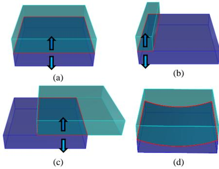
Figure 9. The contact conditions of two CAD models, (a) two equal faces completely contact, (b) two unequal faces completely contact, (c) two faces partially contact, and (d) the contact faces are surfaces.
