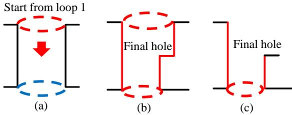
Figure 4. Three kinds of through holes: (a) the side faces evaluated from both loops are identical, (b) the side faces evaluated from both loops are different, and (c) only one loop exists.
