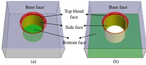
Figure 2. Faces composition of a hole, (a) blind hole and (b) through hole.
