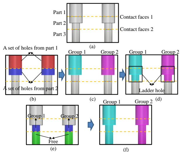
Figure 10. The contact conditions of two CAD models, (a) two equal faces completely contact, (b) two unequal faces completely contact, (c) two faces partially contact, and (d) the contact faces are surfaces.
