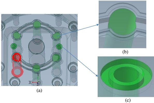
Figure 13. Erroneous holes recognized on CADdoctor, (a) 8 erroneous holes recognized on Part 3 of Case 2, (b) the loop of a hole is cut by other faces, (c) a hole is intersected with a tube.
