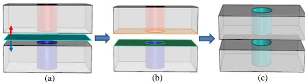
Figure 7. Procedures of detecting related holes across different parts: (a) generate the relationship between parts, (b) search the contact faces, and (c) generate the relationship of holes across different parts.
