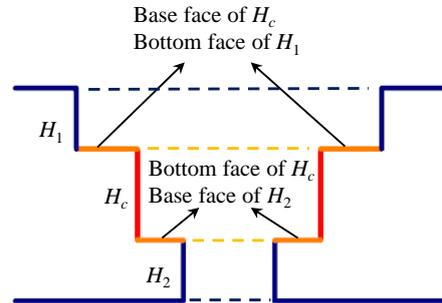
Figure 5. Relationship between neighboring holes, where the hole  $H_c$  neighbors holes  $H_1$  and  $H_2$  with its base and bottom faces, respectively.
