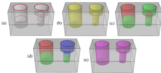
Figure 3. Hole recognition procedures, (a) input loop data, (b) search faces composition on each hole, (c) compute type and associated properties of each hole, (d) detect related holes on each CAD model, and (e) detect related holes across different CAD models.
