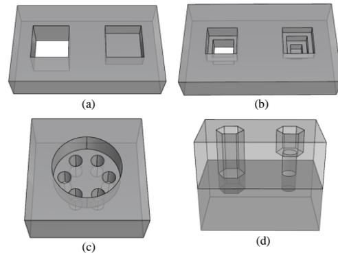
Figure 1. Classification of hole features for feature recognition and simplification, (a) single hole, (b) ladder hole, (c) parallel hole structure, and (d) related holes across different components.
