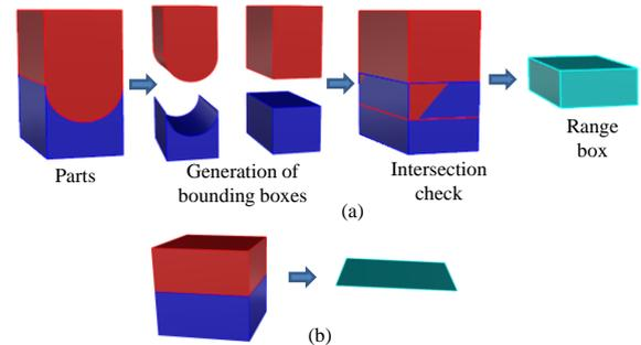
Figure 8. Determine the range box of two intersected CAD models, (a) evaluate the range box of two CAD models, and (b) the range box is reduced to a plane when two CAD models contact at a plane.
