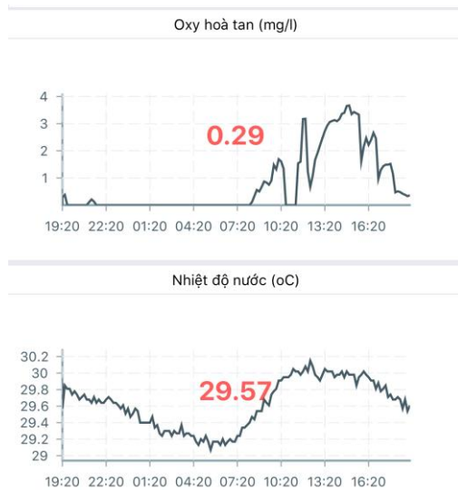
Figure 9. Typical graphs showing dissolved oxygen and temperature parameters.
