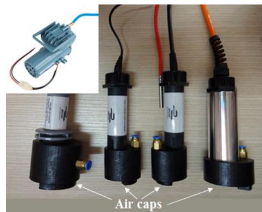
Figure 7. Sensor probes with air caps attached and air pump (small image).
