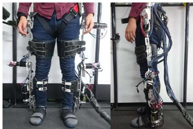
Figure 1. Lower-limb exoskeleton robot.
