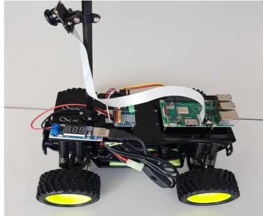
Figure 7. The autonomous car-like mobile robot platform.
