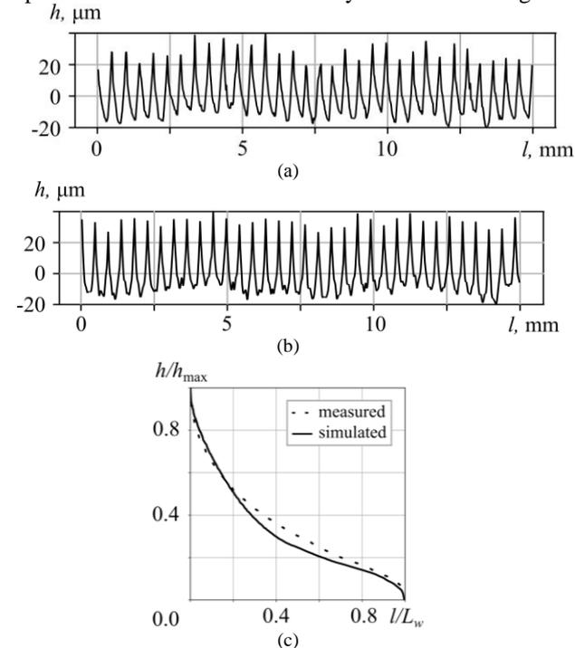
Figure 7. A profile example of measured (a) and simulated (b) planned surfaces and their bearing area curve (c).
