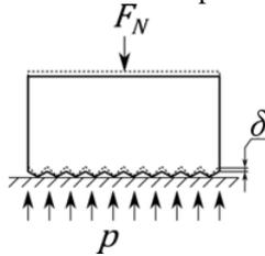
Figure 1. Physical model of contact convergence.
