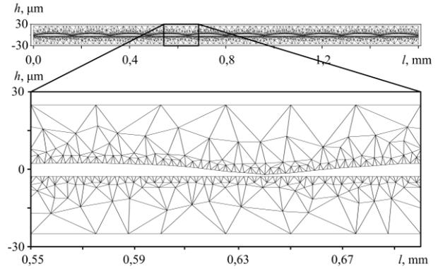
Figure 8. Example of a representative cell of the contact layer
