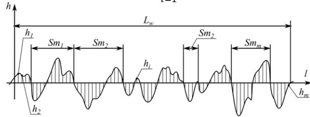
Figure 2. Illustration of calculation of roughness parameters
