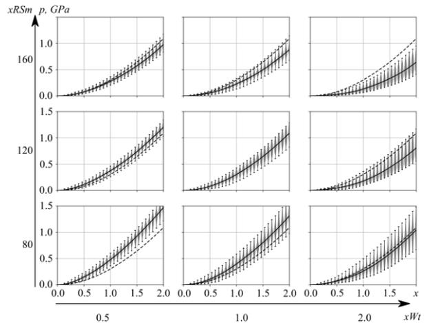
Figure 10. Calculation results of the average elastic characteristics of the contact layer (dashed line – characteristic obtained with  $xWt=1.0$  and  $xRSm=120$ )
