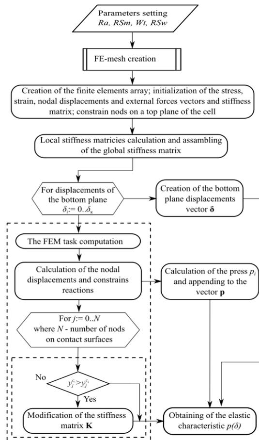
Figure 6. Flow chart of the contact layer elastic characteristic determination algorithm.
