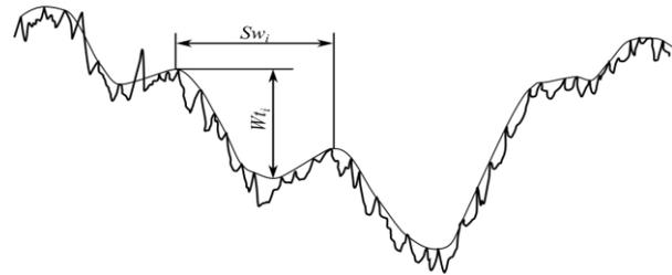
Figure 3. Illustration of calculation of waviness parameters
