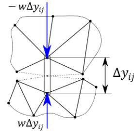
Figure 5. Illustration of multi-point constraints applying.
