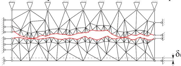
Figure 4. Calculation scheme of the considered contact problem.
