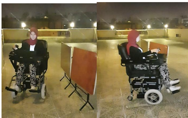
Figure 9. Testing the smart wheelchair motion in case of left obstacle while the joystick motion is go left from the middle of the obstacle.
