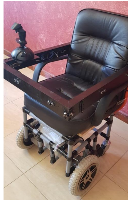
Figure 4. The wheelchair design with all the assembled components
