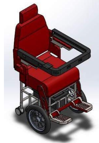
Figure 2. The wheelchair design assembly on SOLIDWORKS
