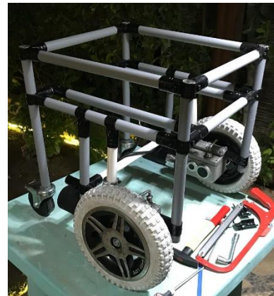
Figure 3. Chassis assembly with drive motors, front and rear wheels
