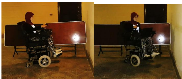
Figure 10. Testing the smart wheelchair motion in case of left and front obstacle while the joystick motion is to go left from the middle of the left obstacle.
