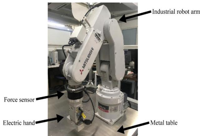
Figure 2. Appearance of industrial robot arm.
