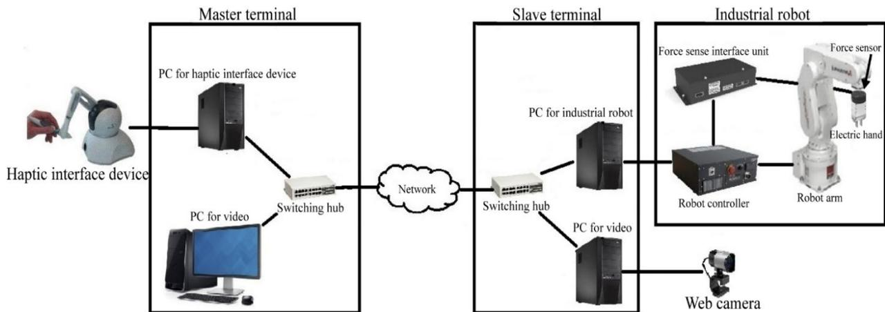
Figure 1. Configuration of remote robot system with force feedback
