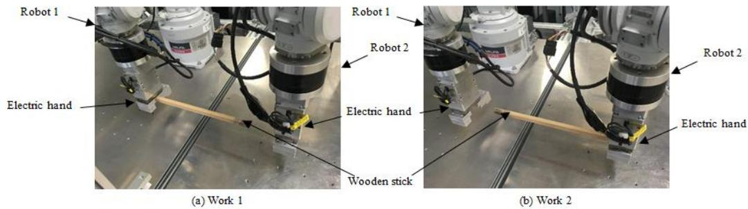
Figure 3. Positional relations of wooden stick between robots 1 and 2.
