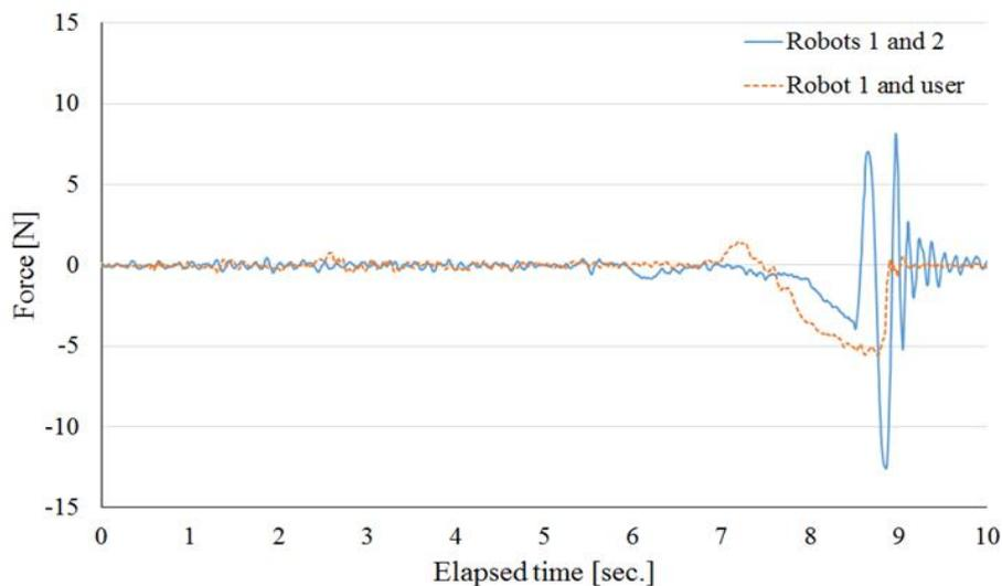
Figure 6. Force of robot 1 versus elapsed time in work 1.
