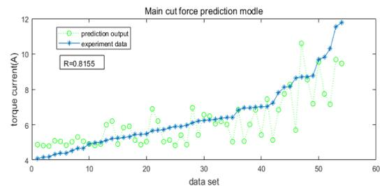
Figure 3. Correlation between the predicted outputs and the experimental data of main cut force
