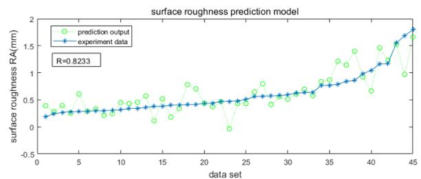
Figure 4. Correlation between the predicted outputs and the experimental data of surface roughness
