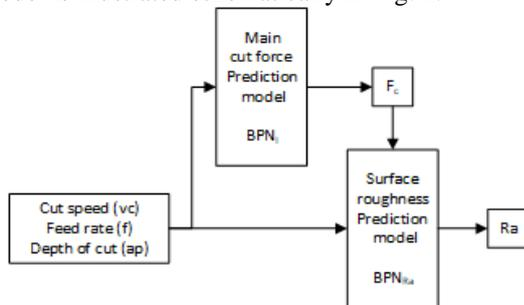
Figure 2. The input/output dataset of the model
