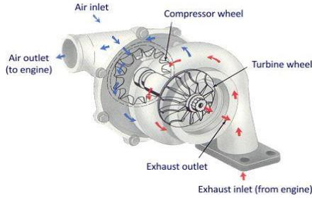
Figure 2. Flow of gasses in a Turbocharger.
