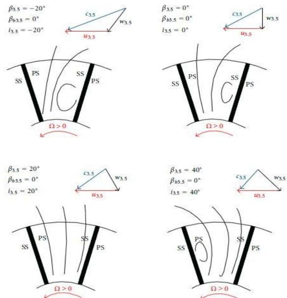
Figure 6. . Velocity diagrams at different relative flow angles.
