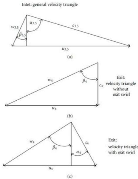
Figure 5. Velocity Triangles at the turbine wheel inlet and exit
