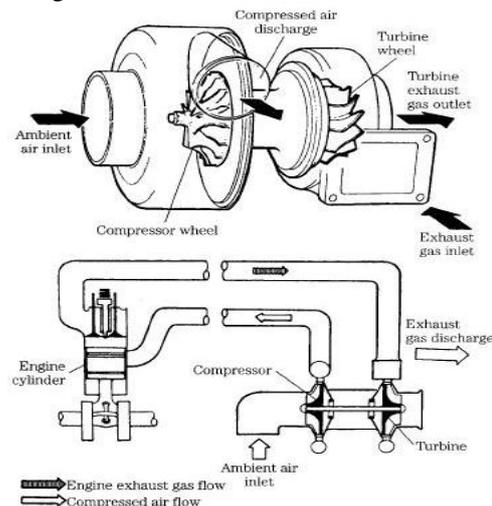
Figure 3. Diesel engine turbocharger
