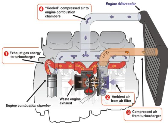
Figure 4. Diesel turbocharged engine system
