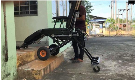
Figure 14. The wheelchair performing stair-climbing.
