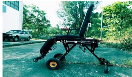
Figure 13a. The designed electric wheelchair.
