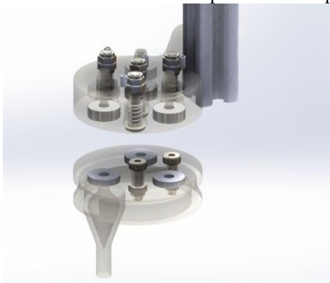
Figure 4. FaRo robot universal tool mount system
