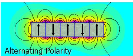
Figure 5. Alternating polarity scheme [9].
