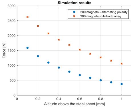
Figure 8. Simulation results for 200 magnets.
