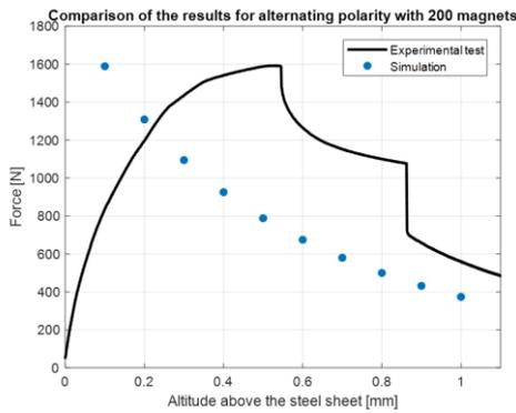
Figure 17. Comparison of the results for alternating polarity with 200 magnets.
