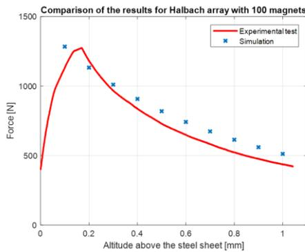
Figure 18. Comparison of the results for Halbach array with 100 magnets.
