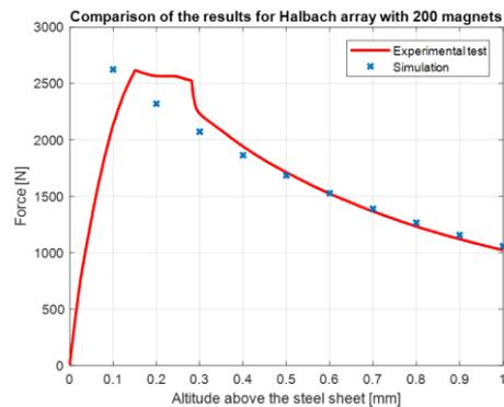
Figure 16. Comparison of the results for Halbach array with 200 magnets.
