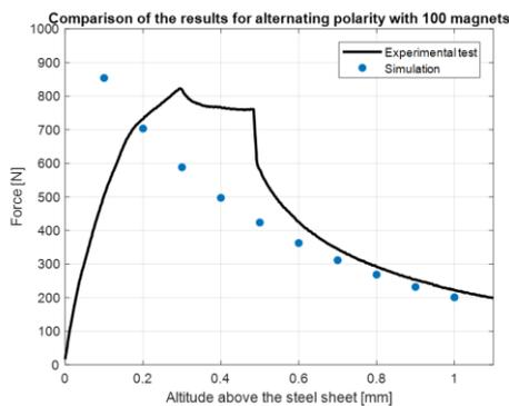
Figure 19. Comparison of the results for alternating polarity with 100 magnets.
