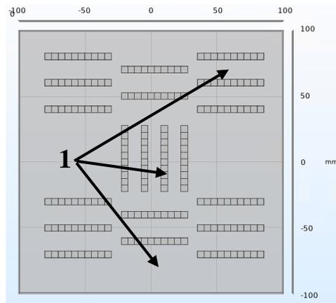
Figure 7. Created system for 200 magnets for the robot floor (1 – magnets).
