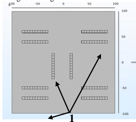
Figure 6. Created system for 100 magnets for the robot floor (1 – magnets).
