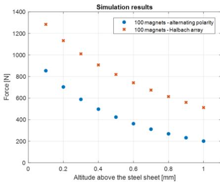
Figure 9. Simulation results for 100 magnets.
