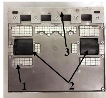
Figure 2. View of the current magnetic system of the MegaSumo robot (1 -magnets; 2 – wheels; 3 - plough).
