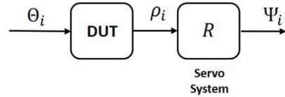
Figure 7. The output of the flex sensors applied on the robotic hand's servo motor system for performance evaluations. The flex sensors are represented by the "DUT" block.
