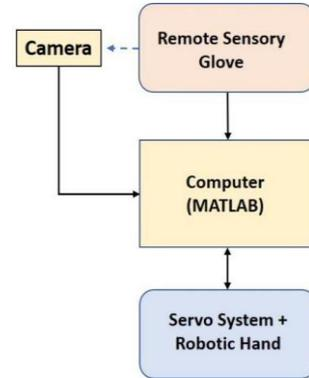
Figure 8. Experimental setup. The camera, robotic hand and the remote sensory glove are connected to a computer for performance evaluation in MATLAB. Black arrows indicate USB connections.
