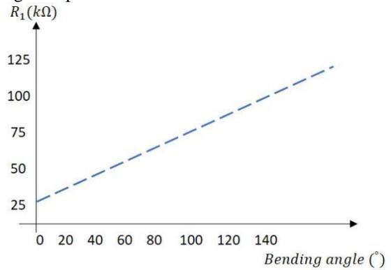
Figure 3. An illustration on the theoretical relationship between  $R_1$  and the sensor's bending angle.
