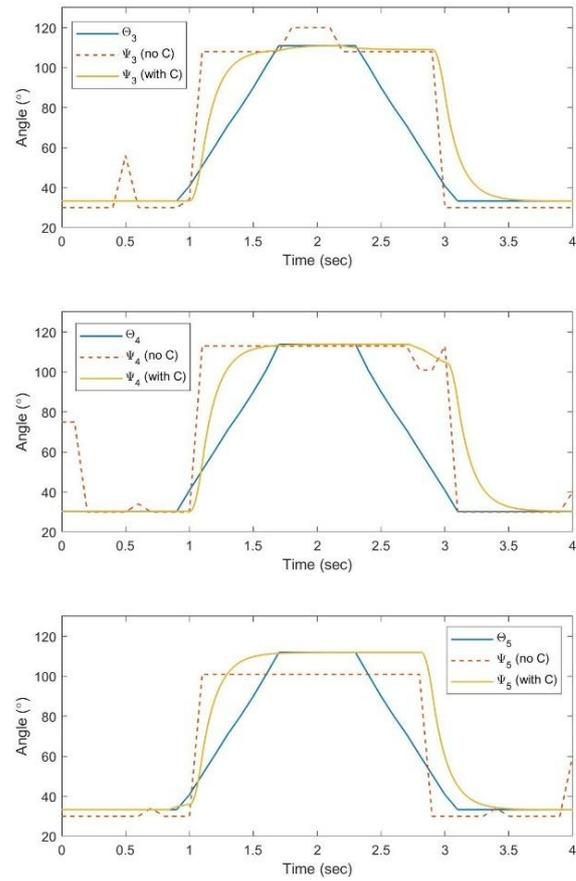
Figure 12. Variations of  $\theta_i$  (in degree) and the corresponding  $\Psi_i$  with compensator (with C) and without compensator (no C) from one of the trials.
