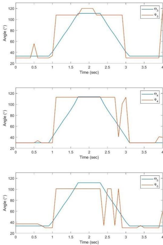
Figure 9. Variations of  $\theta_i$  (in degree) and the corresponding  $\Psi_i$  when there is no compensator for one of the trials.
