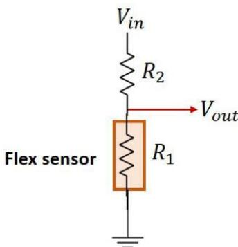
Figure 2. Basic flex sensor circuit.
