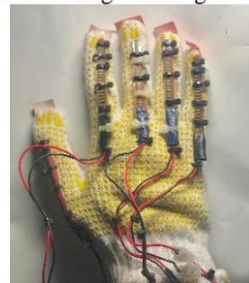
Figure 4. The remote sensory glove.
