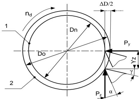
Figure 1. Schematic explaining errors occurring due to forced release of workpiece in a vertical plane under effect of force  $P_z$ .
