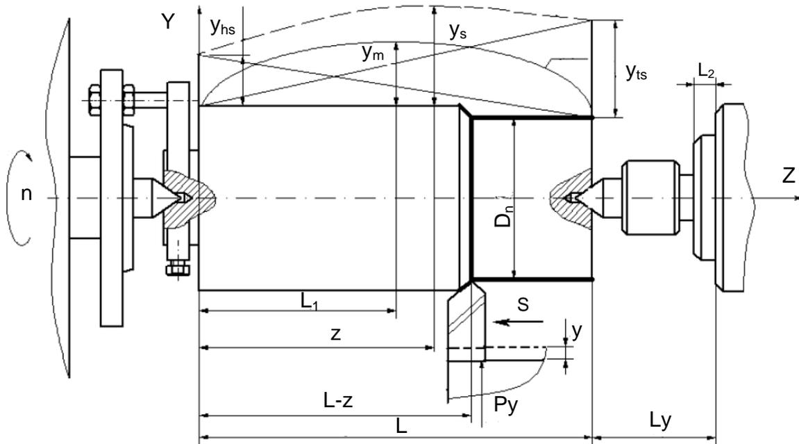
Figure 2. Schematic of formation of errors caused by elastic squeezing of shaft sections under the action of force  $P_y$
