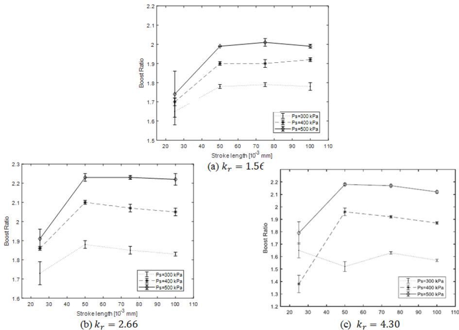
Figure 8. Relation between boost ratio and stroke length.
