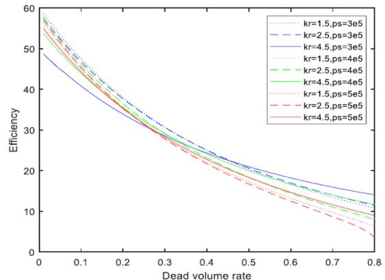
Figure 11. Relationship between the dead volume rate and the energy efficiency.
