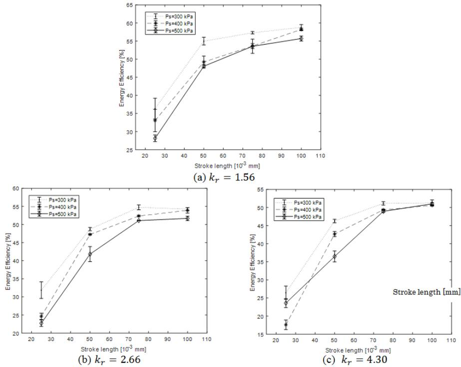
Figure 7. Relation between energy efficiency and stroke length.
