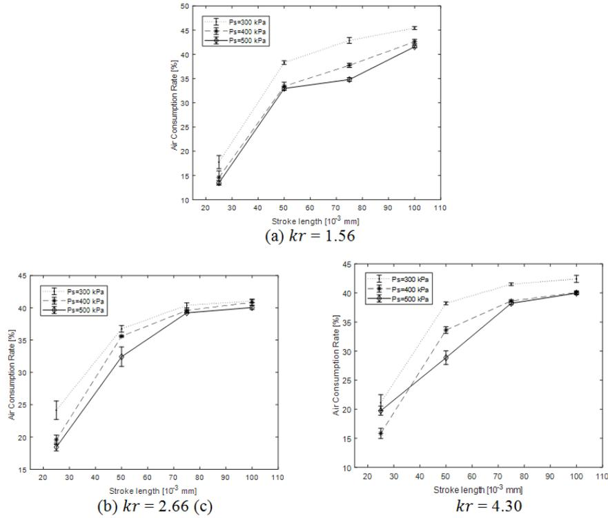
Figure 9. Relation between air consumption rate and stroke length.
