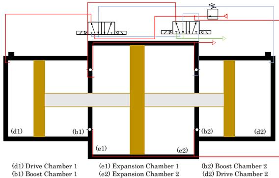
Figure 1. (a) Schematic graphic of PBV-R and (b) principle of PBV-R.
