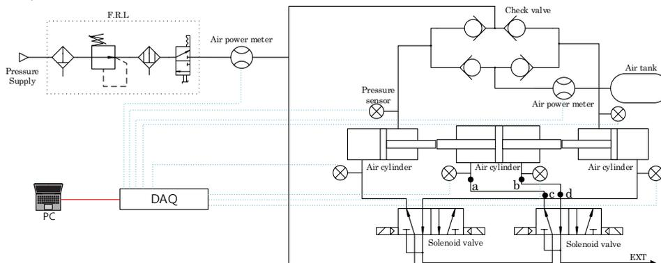
Figure 2. Circuit diagram of PBV-R.
