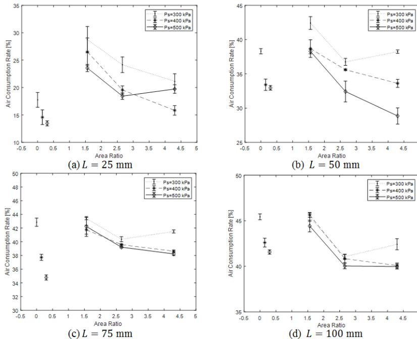
Figure 6. Relation between air consumption rate and area ratio at various stroke lengths.
