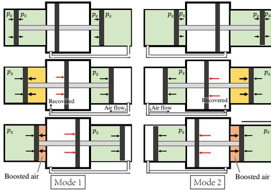
In mode 2, the piston moves to the left. The right side of Fig. 1(b) presents mode 2, and the principle is basically the same as mode 1. Supply air flows into drive chamber 2, boost chamber 1 and 2. For the same reason of mode 1, boost chamber 2 emits air at higher than supply pressure.
