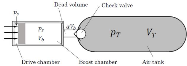
Figure 10. Schematic diagram of a drive cylinder, dead volume and an air tank.
