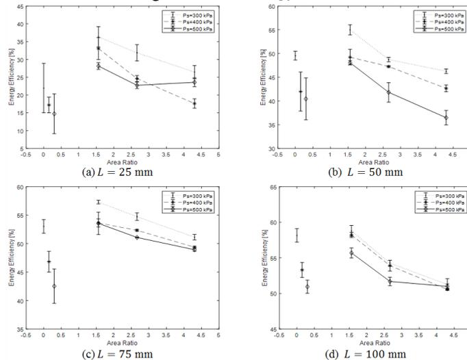
Figure 4. Relations between energy efficiency and area ratio at various stroke lengths.
