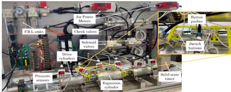
Figure 3. Experimental apparatus of PBV-R.
