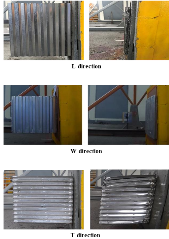
Figure 12. Aluminium honeycomb condition, before and after impact test
