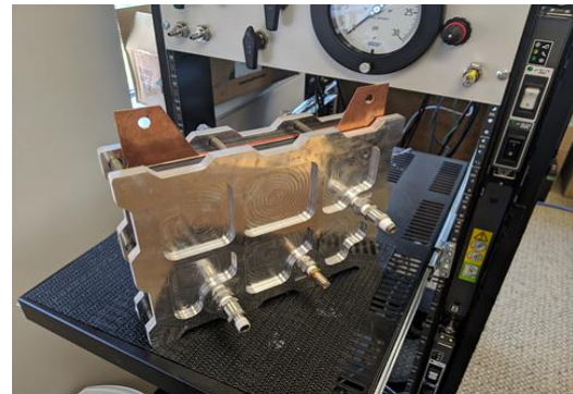
Figure 9. 250 W, 166 cm^2 active area high temperature PEM fuel cell stack on test stand.
