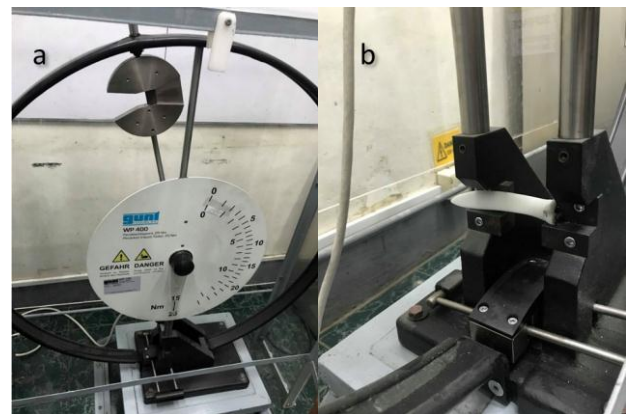
Figure 5. Charpy impact testing apparatus (a) and a propeller specimen loaded in the testing device (b).
