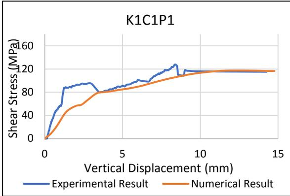
Figure 6. Shear stress-vertival displacement from experimental and numerical modelling for K1C1P1 analysis case
