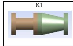
Figure 2. Geometry of male and female components of shear key K1
