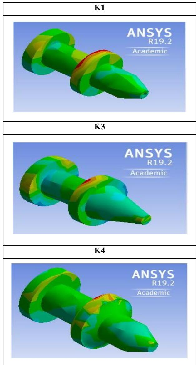
Figure 9. Shear-stress contour in male part at C1P3 case
