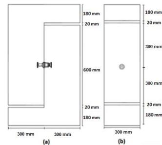
Figure 3. Dimensions of concrete blocks and location of shear key (a) Front view (b) Cross section
