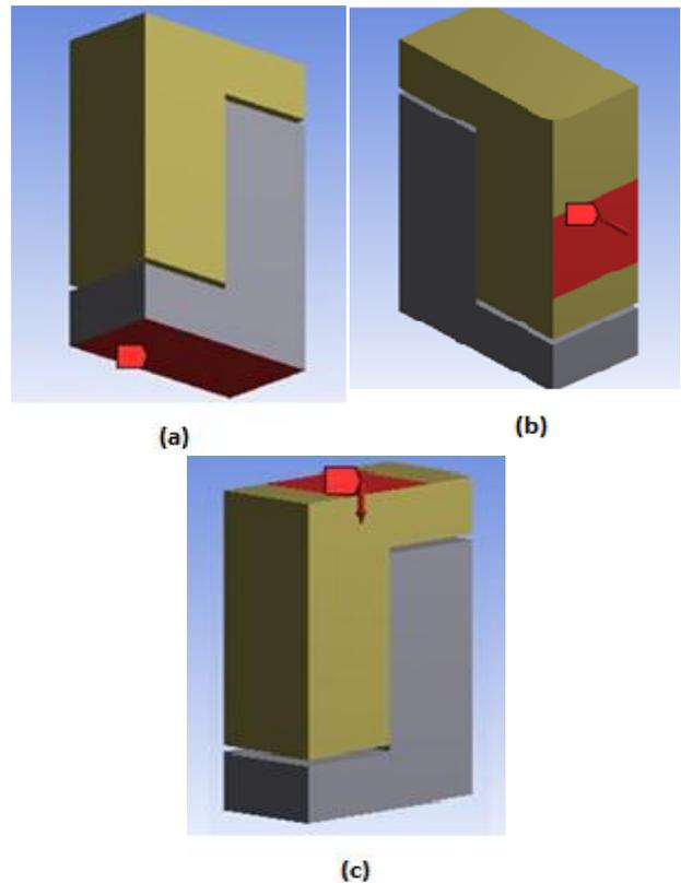
Figure 5. Support condition and loading area: (a) Support, (b) Area of horizontal loading, (c) Area of vertical loading
