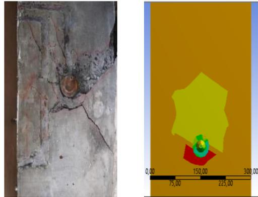
Figure 11. Crack at concrete block near male part at K1C1P1 case
