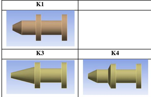
Figure 4. Geometry of three different steel shear keys
