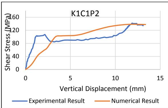
Figure 7. Shear stress -vertival displacement from experimental and numerical modelling for K1C1P2 analysis case
