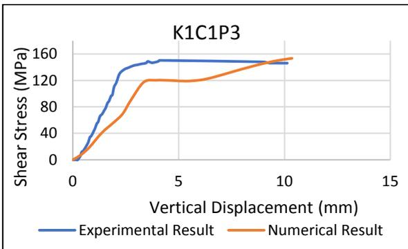
Figure 8. Shear stress-vertival displacement from experimental and numerical modelling for K1C1P3 analysis case
