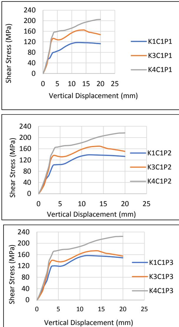
Figure 10. Shear stress-vertical displacement relations for different shear-key geometries, concrete strength, and equivalent prestressing forces
