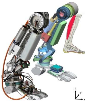
Figure 2. Lower leg - ankle joint - foot - assembly: Next to the biological inspiration (in the back), the CAD-model (middle) depicts the developed lower leg structure, whereas a photograph of the lower leg and ankle joint with the foot is shown in the front.
