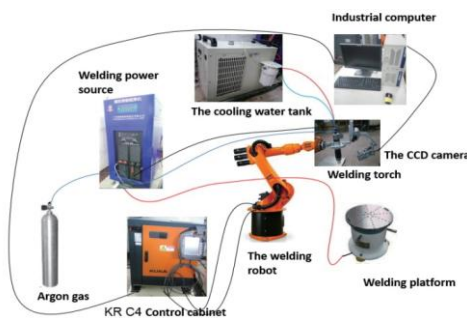
Figure 2. Principle of deep penetration TIG welding [9].
