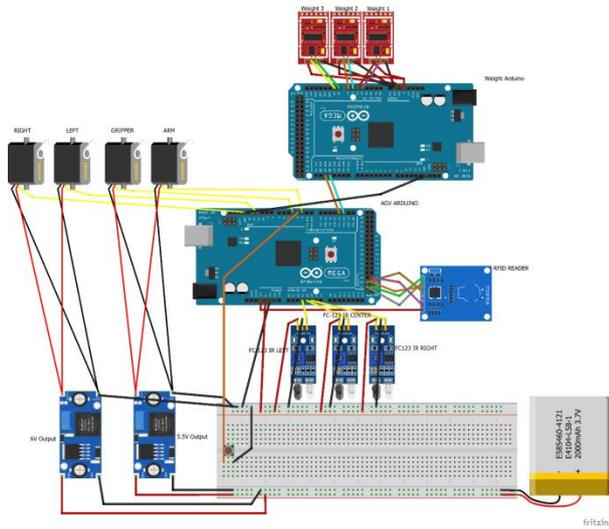
Figure 8. Wiring diagram for the robotic stacker.
