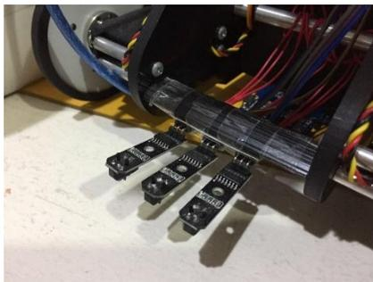
Figure 3. FC-123 line following infrared sensors.
