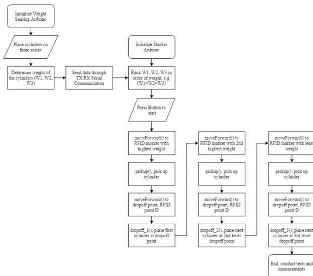
Figure 9. Programming flowchart for the stacking operation.
