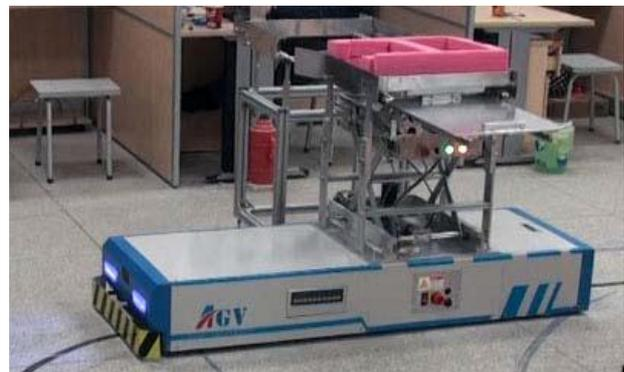
Figure 1. Material transport AGC using electric push rod [2].
