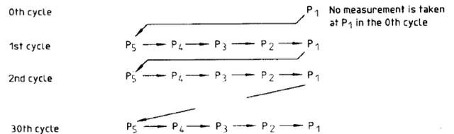
Figure 5. Cycle order for arm-gripper testing [8].
