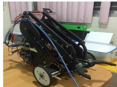
Figure 11. Robotic stacker prototype.
