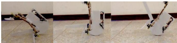
Figure 9. Propeller without protection ring: sometimes it turned successfully.
