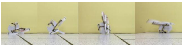
Figure 10. Propeller with protection ring: completed flip
